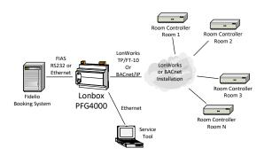
PFG4000 monitors the room status via the Fidelio hotel booking system and informs the HVAC system in the room of the status. In this way it is possible to optimize the energy consumption and comfort by utilize different algorithms in the HVAC system depending on the room status is occupied or unoccupied.
